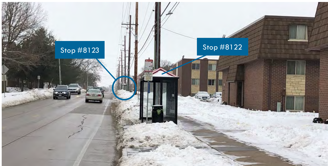
Figure 10-6 Stops Spaced Approximately 500 Feet Apart on W Benton Street
